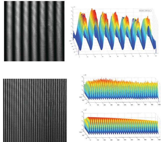
**Figure 10.** Interference pattern and fitting function for different angles between the two surfaces: respectively 150  $\mu\text{rad}$  and 710  $\mu\text{rad}$ .
