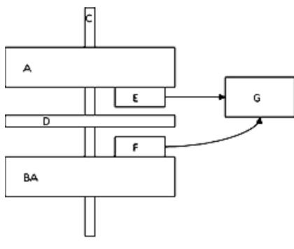
**Figure 1.** Schematic of the rotating encoder principle. D continuously rotating optical encoder; F: reading head fixed to the reference frame BA; E: reading head fixed to the measuring table A; G: phase measurement; C common rotation axis.
