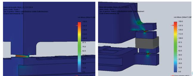
**Figure 7.** A detail of the finite element analysis used for the sizing of the helastic hinges.
