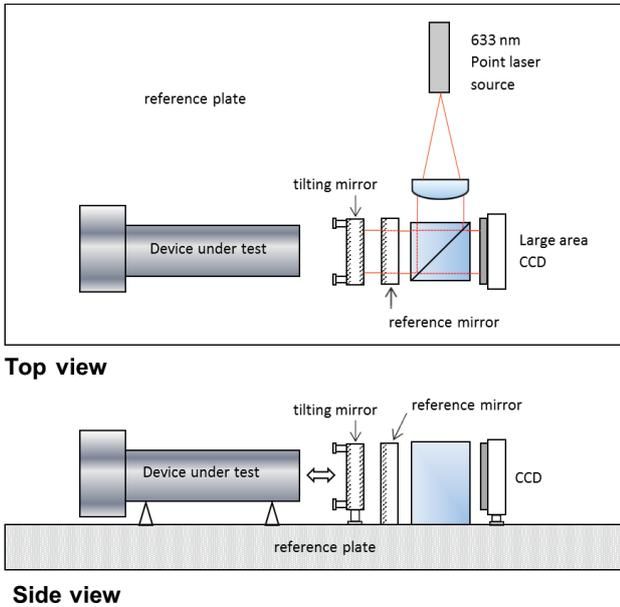
**Figure 8.** Schematic of the FAI. A parallel laser beam is sent to the Fizeau interferometer made of a semi-reflective reference mirror and a mirror which tilt will be measured. The interference pattern is then sent to a calibrated CCD matrix. The ratio between the laser half wavelength and the fringe pitch gives the angle in radian unit.
