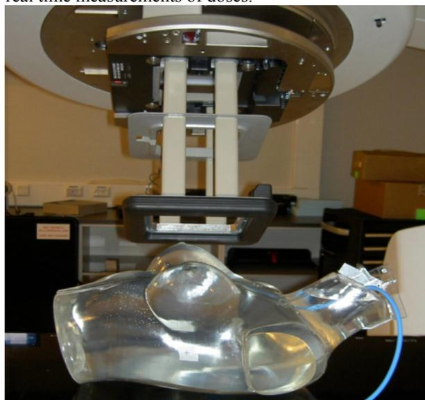
**Figure 7.** STUK prototype of a female torso phantom, internal organs (lung and bone) and computer control of detector movements inside the phantom will be added.
