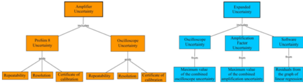
Figure 8: Diagram for ECG simulators uncertainty calculations.
