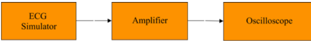
(b) Block diagram for the calibration method of ECG simulators created by Etalons.
