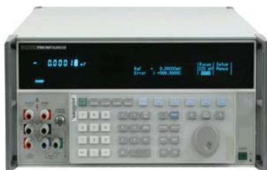
Figure 3. Multifunction calibrator J. Fluke mod. 5700A under calibration in the comparison.
