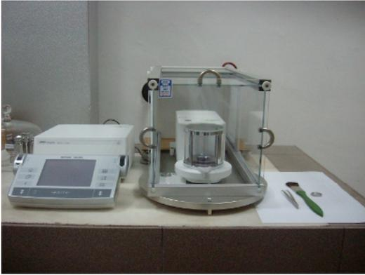
Figure 1. Mass comparator used in calibration
