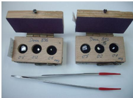
Figure 2. Boxes containing micro masses foil shape
